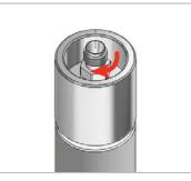
2. Screw the Fitting Body into the end of the stopper assembly (finger-tight).
