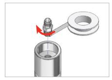
1. Wrap the provided PTFE thread sealing tape around the Fitting Body threads.
