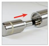
2. Feed the probe of the data logger through the bottom end of the lid.
