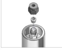
4. Insert the Compression Ferrule into the Fitting Body and hold it in place loosely with the Dome Nut.
