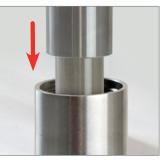
4. Slide the data logger and lid back into the barrier body and screw the lid back on tightly.
